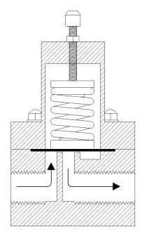
The valve is shipped with a factory set pressure of 100 psig. The diagram to the left shows a cut away view of the position of the diaphragm on the seat.
